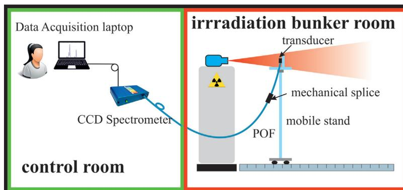
**Fig. 1.** Scheme of the arrangement use for irradiating the fabricated devices. The transducers are placed normal to the beam propagation of the gamma radiation, and the distal end of the fiber, located at the control room, is attached to a commercial CCD spectrophotometer and a laptop.
