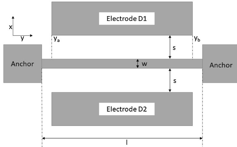
**Fig. 1.** Schematics of a cc-beam showing the geometrical parameters: length ( $l$ ), width ( $w$ ) and beam-driver gap distance ( $s$ ). The thickness ( $t_h$ ) dimension is normal to the plane  $x$ - $y$ . Material properties are determined by Young modulus ( $E$ ) and mass density ( $\rho$ ).
