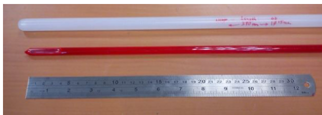
Fig. 1. (a) Photo showing the constituents of the glow-stick: (top most) outer plastic tube and (middle) the inner glass tube containing diphenyl oxalate in red dye. (For interpretation of the references to colour in this figure legend, the reader is referred to the web version of this article.)
