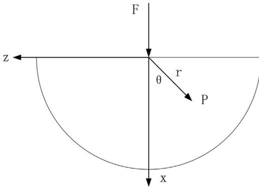
Fig. 1. Semi-infinite plane subjected to radial force.
