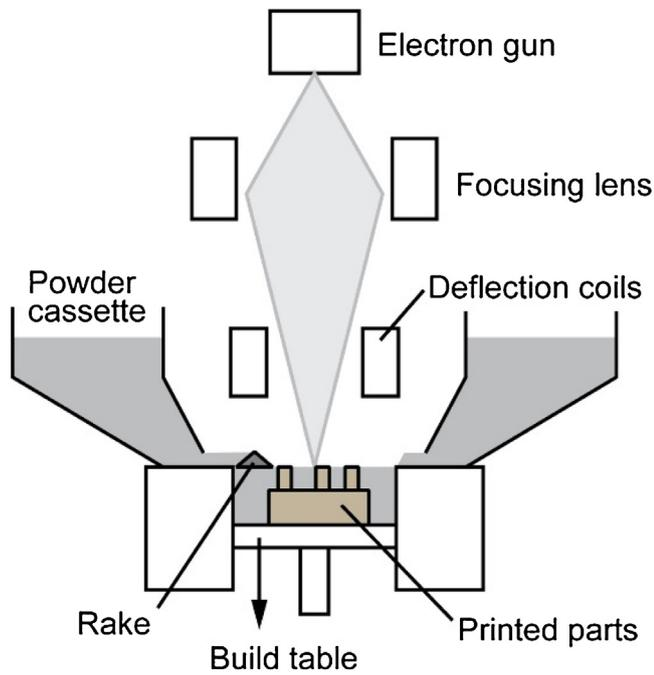
**Fig. 1.** The diagram of additive manufacturing based on Electron Beam Melting (adapted from [1]). The Focused electron beam in a vacuum chamber scans the titanium alloy powder layer by layer to directly “print” 3D parts.
