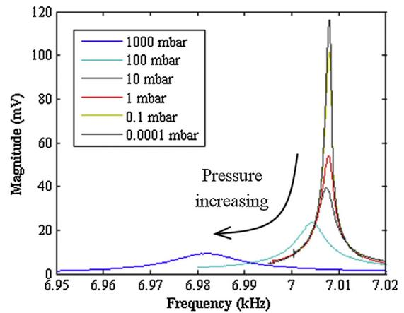
Fig. 3. Resonant measurements of the cantilever under different pressures in  $\text{N}_2$  environment for the first flexural mode.
