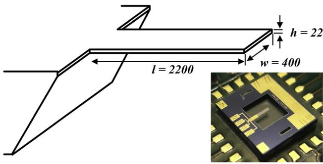
Fig. 1. Schematic diagram and photo of the piezoelectric microcantilever with all dimensions given in  $\mu\text{m}$ .
