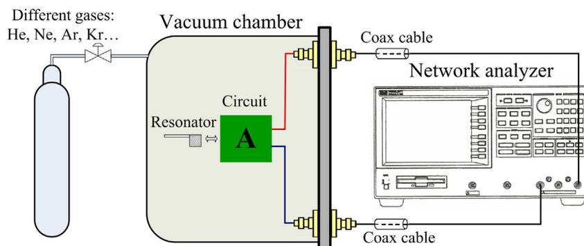
Fig. 2. Schematic diagram of the measurement setup.
