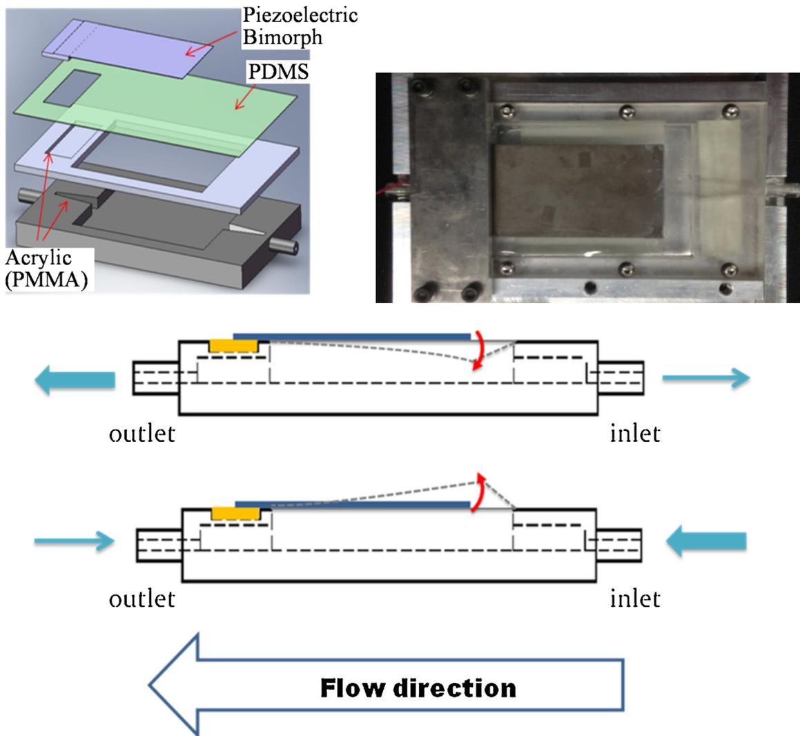
Fig. 1. The configuration and operating characteristics of piezoelectric hydroacoustic using piezoelectric bimorphs and PDMS membrane (Type A).
