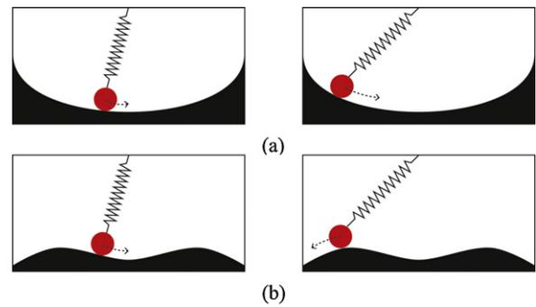
Fig. 1. Metaphors of magnetic systems: (a) linear resonant actuator and (b) linear impact resonant actuator.
