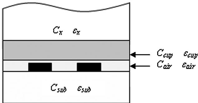
**Fig. 3.** Cross-section view of IDC sensor with its superimposed layer capacitance configuration.
