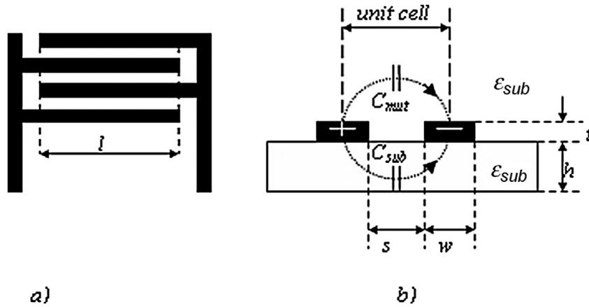
**Fig. 1.** IDC: (a) planar structure, (b) cross-sectional view ( $l$  – length of the fingers,  $h$  – height of the substrate used,  $t$  – thickness of the conductive material forming electrodes,  $\epsilon_{sub}$  – permittivity of substrate,  $\epsilon_x$  – permittivity of MUT,  $s$  – electrode spacing,  $w$  – electrode width).
