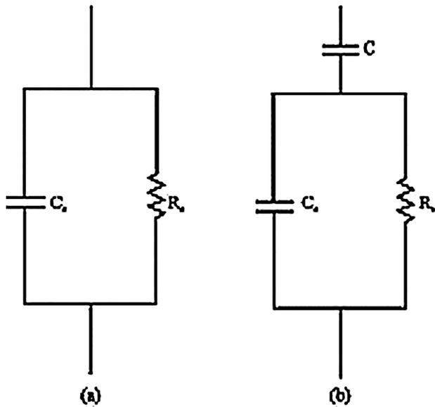
**Fig. 2.** Equivalent circuits for: (a) invasive and (b) non-invasive electrode arrangement.
