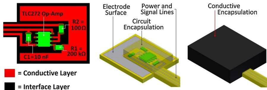
Fig. 1. Active electrode circuit (left) and structure (middle and right).
