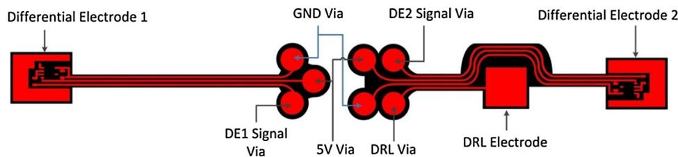
Fig. 2. A three electrode layout for a one-lead bipolar ECG chest band using active electrodes.
