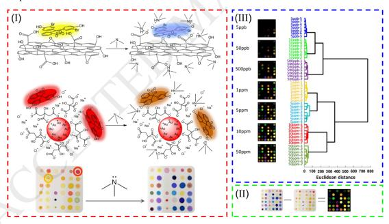
**Abstract Graphic:** (I) The reaction between the array fabricated from nanocomposites and TMA; (II) The generation of difference map; (III) Ultrasensitive detection of TMA among the concentrations from 5 ppb to 50 ppm.
