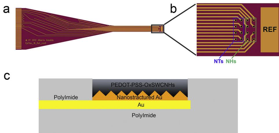
Fig. 1. a) Representative scheme of the whole  $\mu$ EcoG array used for neural signal recording, b) details on the position of NTs and NHs coatings on electrodes and c) scheme of the NHs modified microelectrode.
