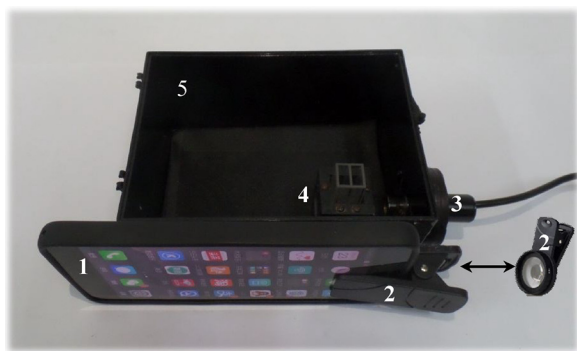
Fig. 1. Schematic illustration of the double-channel smartphone-based RLS detection device for portable analysis. (1) smartphone, (2) macro lens, (3) laser pointer, (4) twin cuvette and frame; (5) black box.
