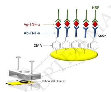
Schematic illustration of the electrochemical cell and the modified immunosensor surface with a sandwich type Ab-TNF- $\alpha$ @HRP-- Ag-TNF- $\alpha$  -- Ab-TNF- $\alpha$
