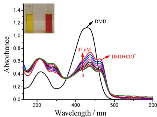
**Fig. 1.** UV-vis spectra of DMD (10 mM) (black line) and DMD (10 mM) with hypochlorite (0–45 nM) in DMSO–water solution (1: 1, v/v, 50 mM PBS buffer solution at pH 7.4). Inset: images of DMD (canary yellow, left) and in the absence  $\text{OCl}^-$  under day light (gules, right). (For interpretation of the references to colour in this figure legend, the reader is referred to the web version of this article.)
