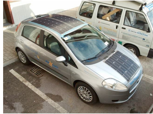
Fig. 2. Hybrid Solar Vehicle by University of Salerno
