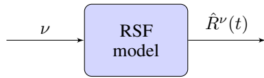
Fig. 1. A random survival forest computes the maximum likelihood estimate \hat{R}^\nu(t) of the reliability function given a vehicle represented by the data \nu . With the estimate \hat{R}^\nu(t) , the battery lifetime prediction function \mathcal{B}^\nu(t; t_0) in (2) can be computed.
