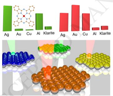
Sensing applications with surface-enhanced Raman spectroscopy (SERS) can benefit from aluminum and copper. Self-assembled monolayers of nanospheres coated with copper and aluminum films produce controlled plasmonic nanostructures. When all other parameters are kept constant, copper and aluminum are found to be at the same level of SERS performance as nanostructures made with silver or gold. This finding opens the door to inexpensive large-scale development of SERS sensors.
