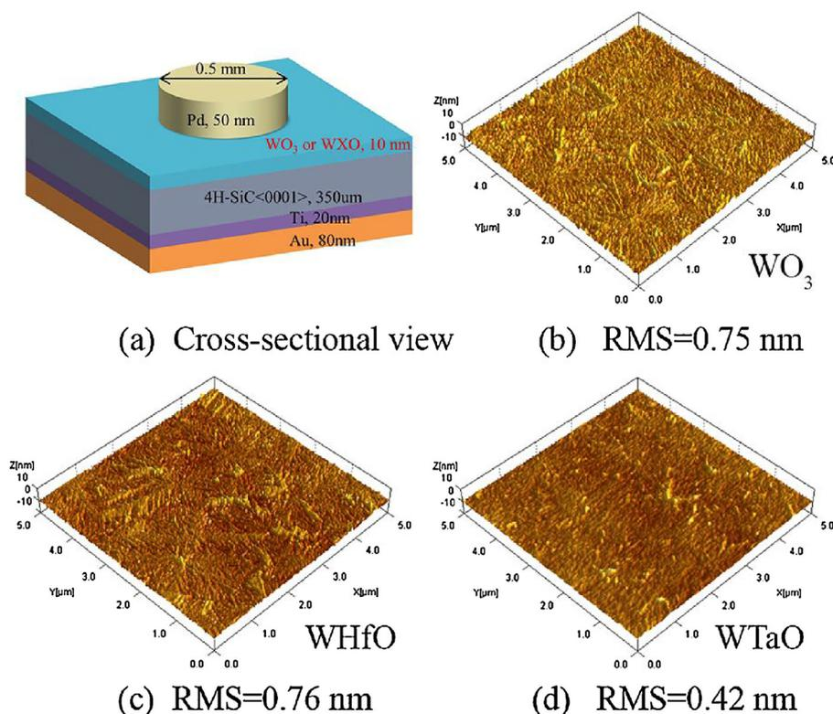
Fig. 1. (a) Cross-sectional view of Schottky-diode gas sensor. AFM image with a measurement area of  $5 \mu\text{m} \times 5 \mu\text{m}$ : (b)  $\text{WO}_3$ , (c)  $\text{WHfO}$ , (d)  $\text{WTaO}$ .
