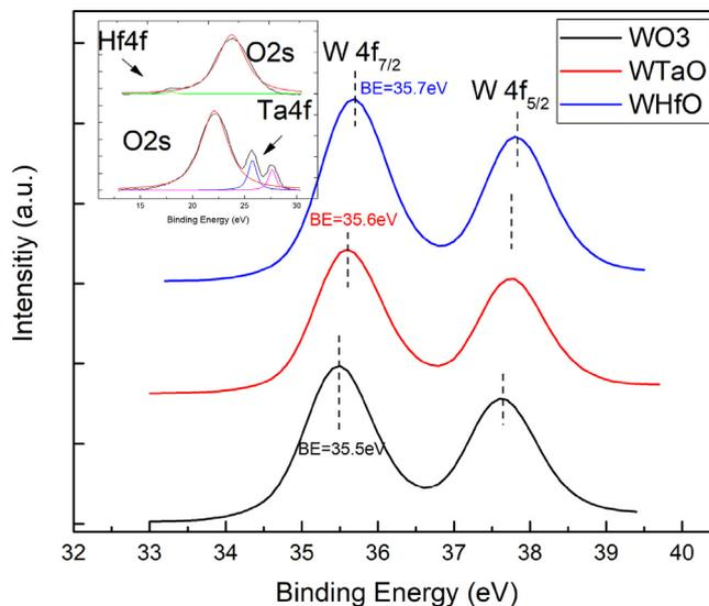
Fig. 2. XPS core-level W 4f and O 2s (inset) spectra of the nanostructured oxide films.
