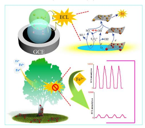
Scheme 1. Schematic for the ECL of TCPP NS-GO/K<sub>2</sub>S<sub>2</sub>O<sub>8</sub> system with sensitive detection of Fe<sup>3+</sup>.
