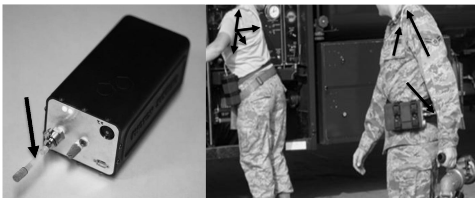
Fig. 1. (Left Panel) Picture of the NaDos, showing the ruggedized black ABS shell, Inlet and outlet ports and indicator LED lights, and recessed power/event maker button. (Right Panel) NaDos, being worn in the field by fuel handlers. In this photo, the fuel handlers are wearing the NaDos in both the horizontal and vertical orientations. The air inlet tubes (shown at the tips of the black arrows) terminate in the “breathing zone” to sample equivalent airspace as the workers respiration zone.
