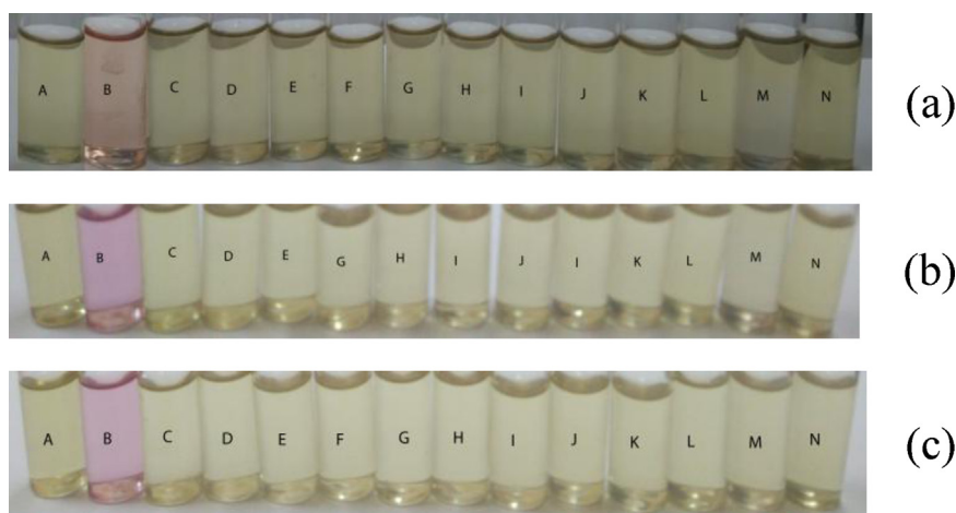
Fig. 2. Color change upon addition of 1.0 equivalent of tetrabutyl ammonium anions into a solution of spiropyran receptor 1 in MeCN: (10 mM HEPES) water (4:6) at (a) pH = 5.0, (b) pH = 7.6 (c) pH = 9.0. [ 1 ] = 2.5 \mu\text{M} . From left to right; A = Free receptor, B = \text{CN}^- , C = \text{F}^- , D = \text{OAc}^- , E = \text{Cl}^- , F = \text{Br}^- , G = \text{I}^- , H = \text{NO}_3^- , I = \text{H}_2\text{PO}_4^- , J = \text{HSO}_4^- , K = \text{PF}_6^- , L = \text{OH}^- , M = \text{S}^{2-} , N = \text{SH}^- .
