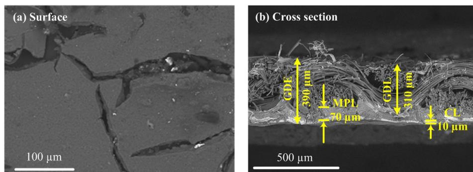
**Fig. 1.** SEM micro porous structure of a typical sensor electrode (a) surface, (b) cross section view.
