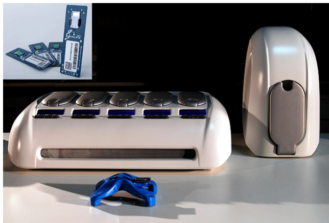
Fig. 2. In-Check platform. Composed by a Thermal Control System (TCS) (on the left) and an optical reader (on the right) based on a CCD camera acquisition system. In the inset is reported the LoC device.
