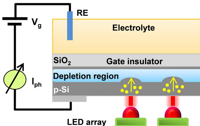
Fig. 1. Schematic of the multi-spot LAPS consisting of an Al–Si–SiO<sub>2</sub> structure and measurement setup. RE: reference electrode;  $I_{ph}$ : photocurrent;  $V_g$ : gate voltage.
