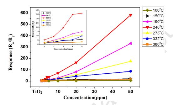
Response of the sensor based on ultralong  $MoO_3$  nanobelts exposure of different concentrations of TMA at different temperatures.
