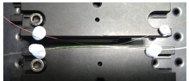
Fig. 2. Detail of the experimental setup showing the translation stages with the fibers attached to them.
