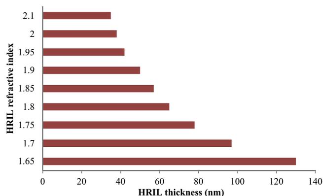
Fig. 2. Correlation between the thickness and the refractive index value of the HRIL in order to maximize the intensity of the EF.
