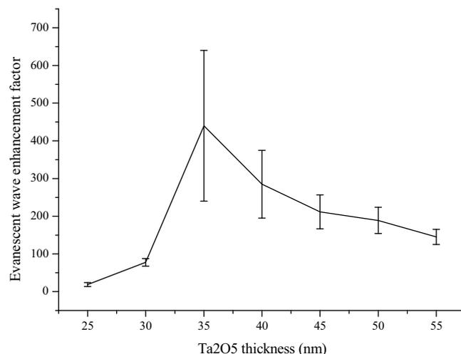
Fig. 3. EF enhancement factor as function of the  $\text{Ta}_2\text{O}_5$  thickness.
