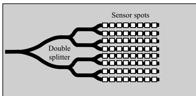
Fig. 1. Design of the multianalyte biosensor platform.
