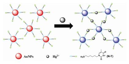
Scheme 1. Schematic illustration of N-T/AuNPs-based colorimetric detection of Hg<sup>2+</sup>.
