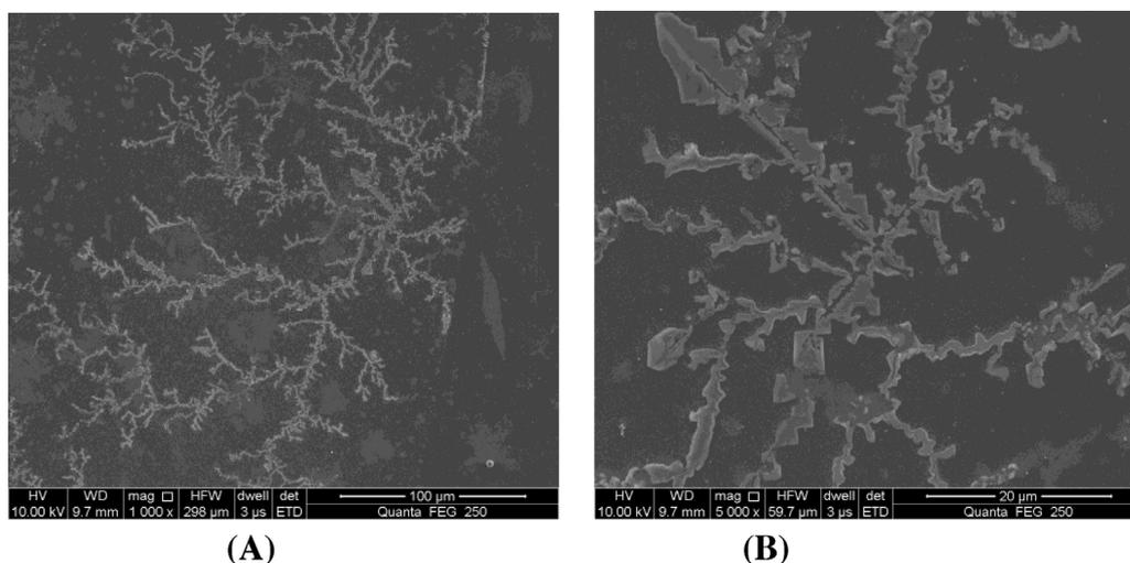
Fig. 1. SEM characterization of the synthesized Pd–Au bimetallic cluster.
