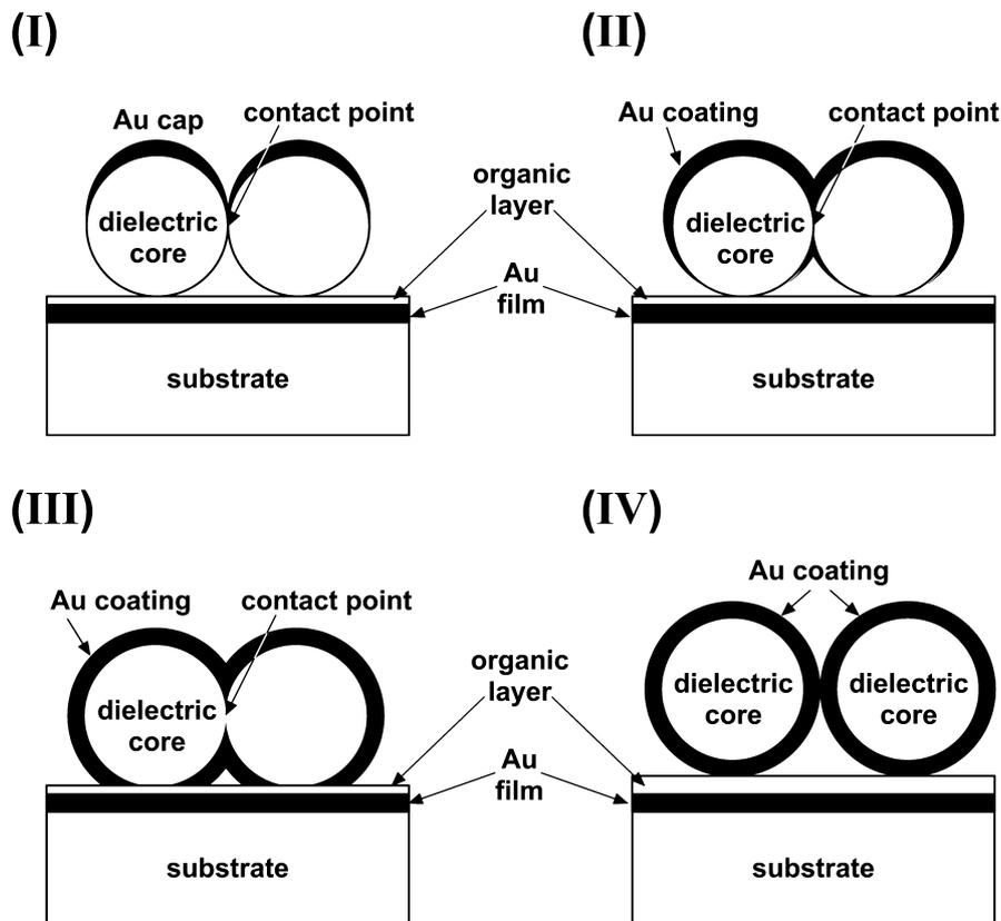
**Fig. 1.** Schemes of the four different hybrid structures studied. Polystyrene (PS) nanoparticles are adsorbed on a thin gold film evaporated on a PS substrate. Subsequently, the PS particles are coated with gold by evaporation (I), sputtering (II), or wet chemistry (III). In the case of (IV), the PS particles were coated with gold by wet chemistry before surface adsorption and therefore do not allow for direct contact points between neighboring dielectric cores.
