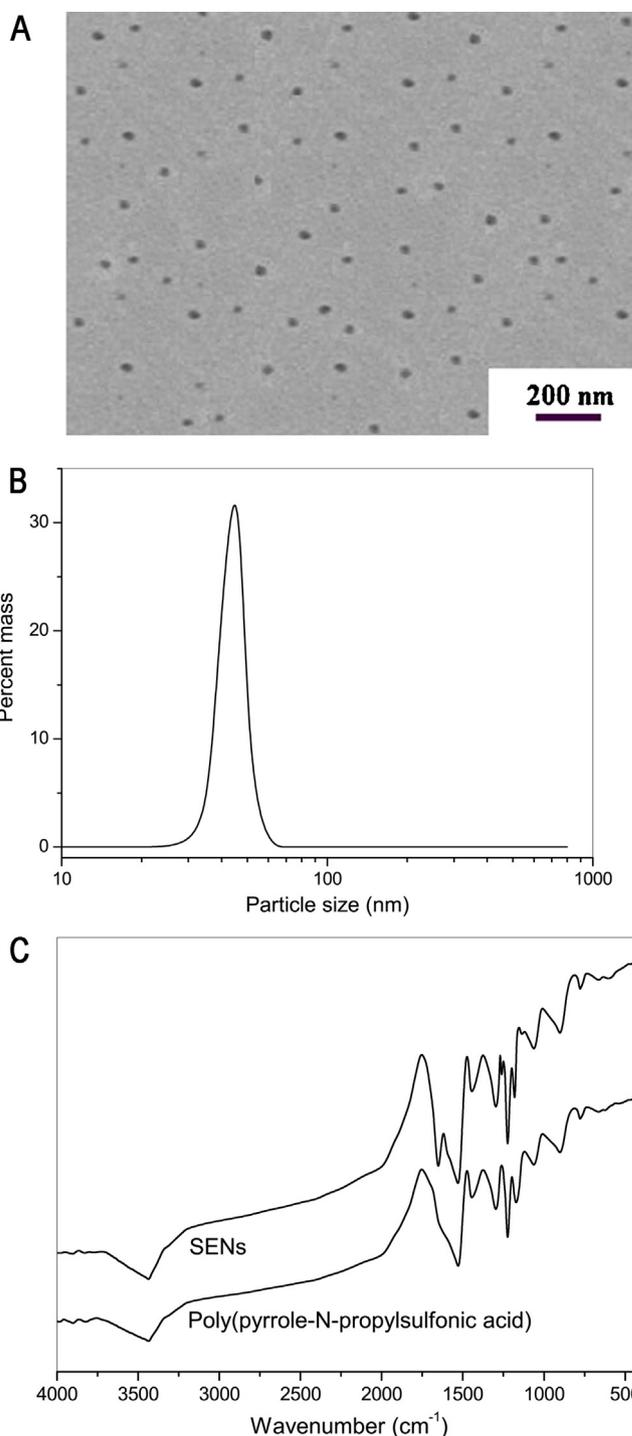
**Fig. 1.** TEM image (A), particle size distribution (B) and FTIR spectra (C) of synthesized SENs.
