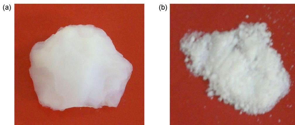
**Fig. 1.** Images of hydrophobic silica aerogel and nano-silicon powder, (a) a piece of hydrophobic silica aerogel, and (b) nano SiO<sub>2</sub> powder.
