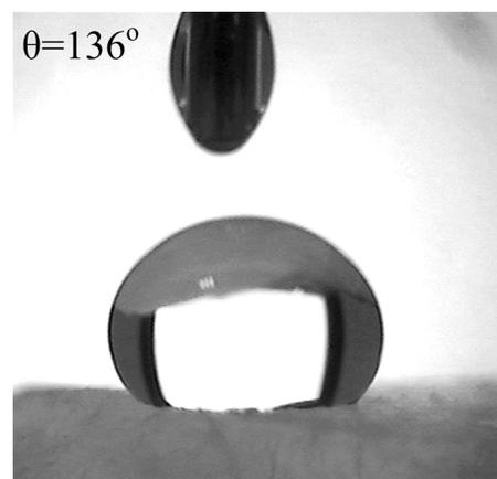
**Fig. 2.** Hydrophobicity of silica aerogel. The contact angle of a water drop on a piece of silica aerogel was measured to be 136°.
