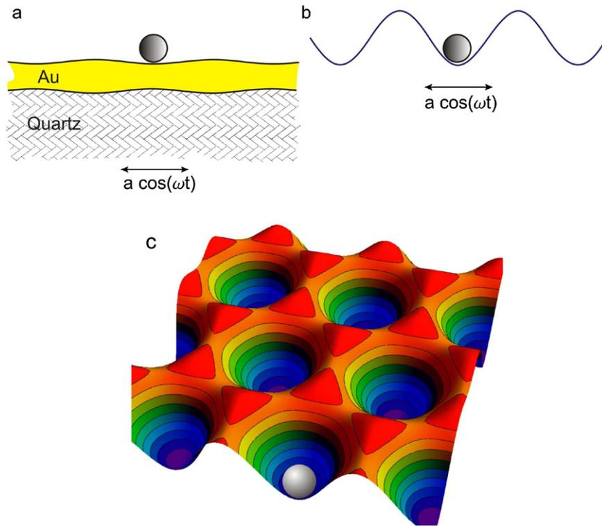
**Fig. 1.** (a) A particle on a gold electrode of a quartz crystal resonator. (b) The particle in a simplified one-dimensional periodic potential of the surface–particle interaction. (c) The particle in a 2D periodic potential of the Au(111) surface–particle interaction, the particle having a single point of contact.
