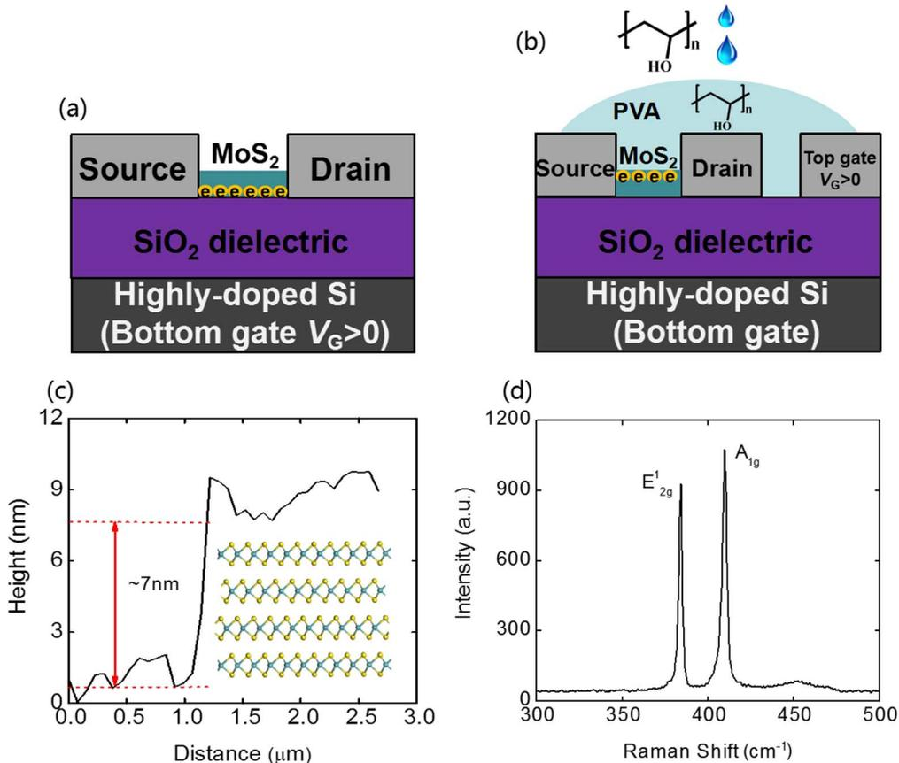
Fig. 1. (a) The schematic cross-section of multilayer MoS<sub>2</sub> transistor. (b) The schematic cross-section diagram of MoS<sub>2</sub> transistor using PVA as dielectric layer. (c) AFM image at the MoS<sub>2</sub> flake edge. (d) The Raman spectroscopy for the MoS<sub>2</sub> flake.
