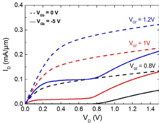
Fig. 1. Output  $I_D(V_D)$  characteristics with back-gate voltage  $V_{Gb} = 0$  and  $V_{Gb} = -5$  V.  $W = 10 \mu\text{m}$ ,  $L = 100$  nm,  $t_{si} = 25$  nm,  $t_{ox} = 2.9$  nm, 25 nm BOX thickness.
