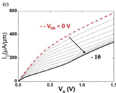
Fig. 2. Impact of back-gate bias  $V_{Gb}$  from 0 V to  $-10$  V (step  $-1$  V) on  $I_D(V_D)$  characteristics for various channel lengths: (a)  $1 \mu\text{m}$ , (b)  $150$  nm, and (c)  $50$  nm;  $t_{si} = 25$  nm.  $V_{Gf} = 1$  V.
