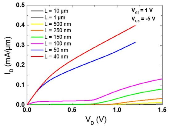
Fig. 3.  $I_D(V_D)$  curves showing the kink effect dependence on channel length.  $W = 10 \mu\text{m}$ .
