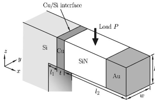
Fig. 1. Schematic illustration of a straight nano-cantilever specimen and its loading method.
