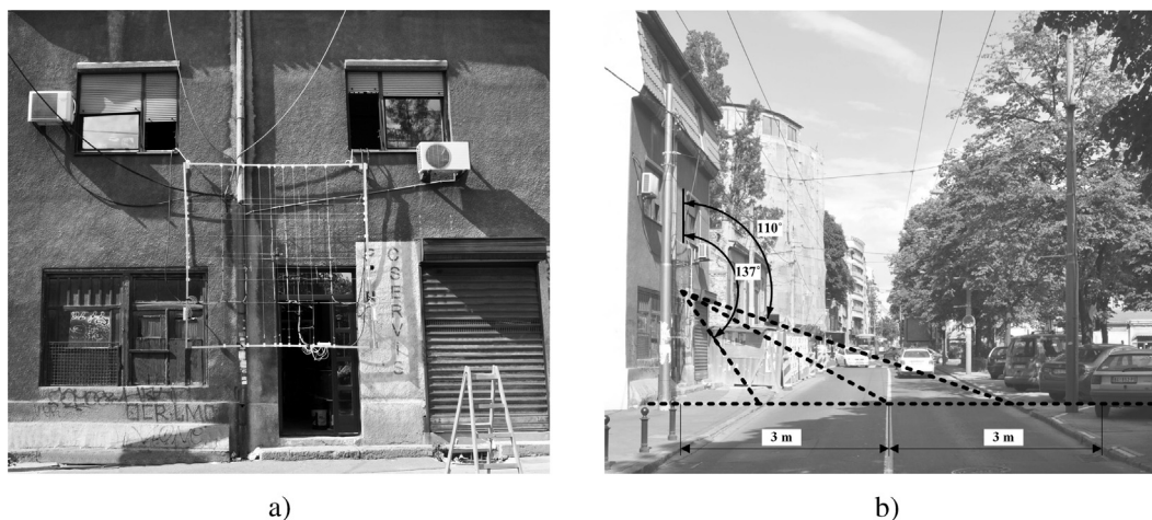
Fig. 1. a) Microphone array on the façade, and b) the profile of the street.
