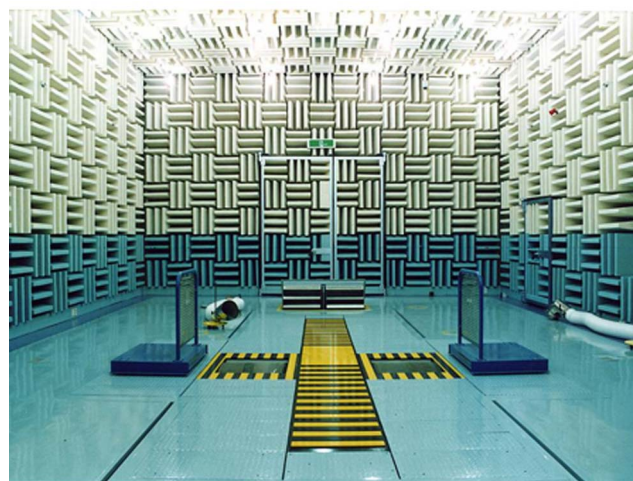
Fig. 1. Semi-anechoic room and dynamometer for sound recording.
