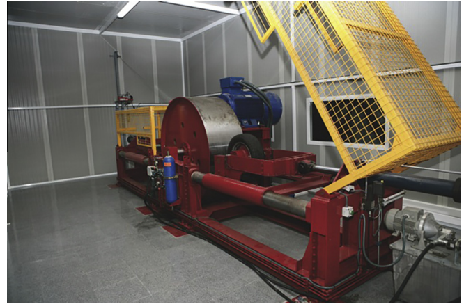
Fig. 1. Research group's drum tyre test facilities.
