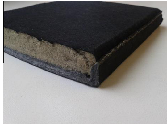
Fig. 2. High absorbing sandwich material of the thermo-acoustic encapsulation.
