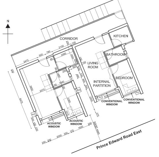
Fig. 1. Layout plan of the mock-up flats (All dimensions in mm).
