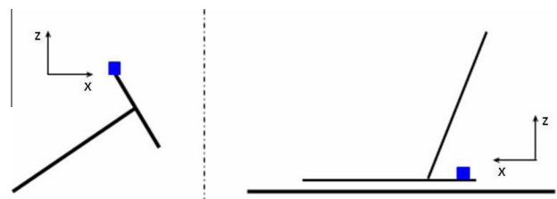
Fig. 1. Locations of the three-axis accelerometers (blue) on the steering-wheel (left side of the figure) and on seat (right side of the figure) during the vibrations' recordings. (For interpretation of the references to color in this figure legend, the reader is referred to the web version of this article.)
