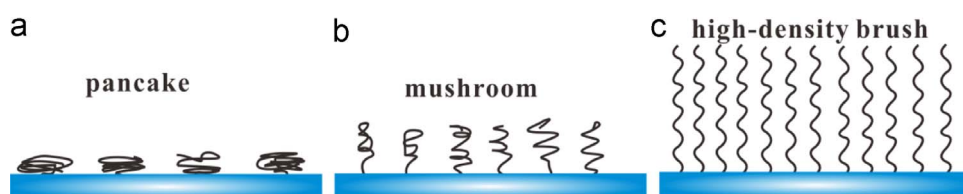
Fig. 1. Schematic illustration of three typical configurations of surface attached polymers with increasing grafting densities.
