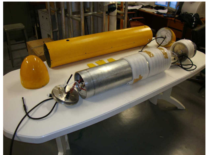
Figure 3. Parts of the hull, main e and manoeuvring vessels
