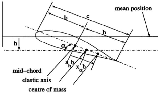
**Fig. 1.** The sketch of an airfoil oscillating in pitch ( $\alpha$ ) direction with respect to the elastic axis, and in plunge ( $h$ ) direction measured from the mean position.
