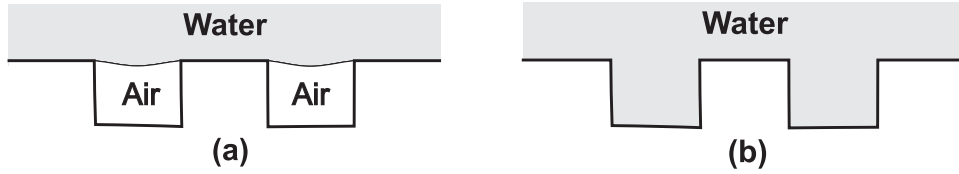
Fig. 1. Schematic of a super-hydrophobic surface. (a) Cassie–Baxter state of super-hydrophobicity with the air trapped into the grooves. (b) Wenzel state of super-hydrophobicity with the water penetrated into the grooves.
