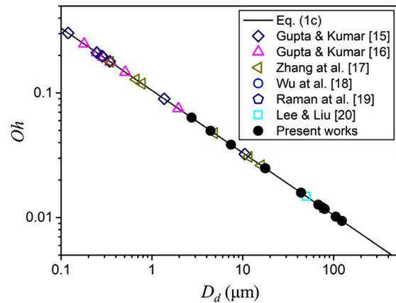
Fig. 1. Summary of LBM studies on water droplet impacting on a solid surface with different  $Oh$  numbers in previous work and present work.
