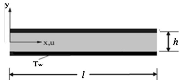
Fig. 1. Schematic of the model problem of a two-dimensional microchannel between two plates with constant wall temperature.
