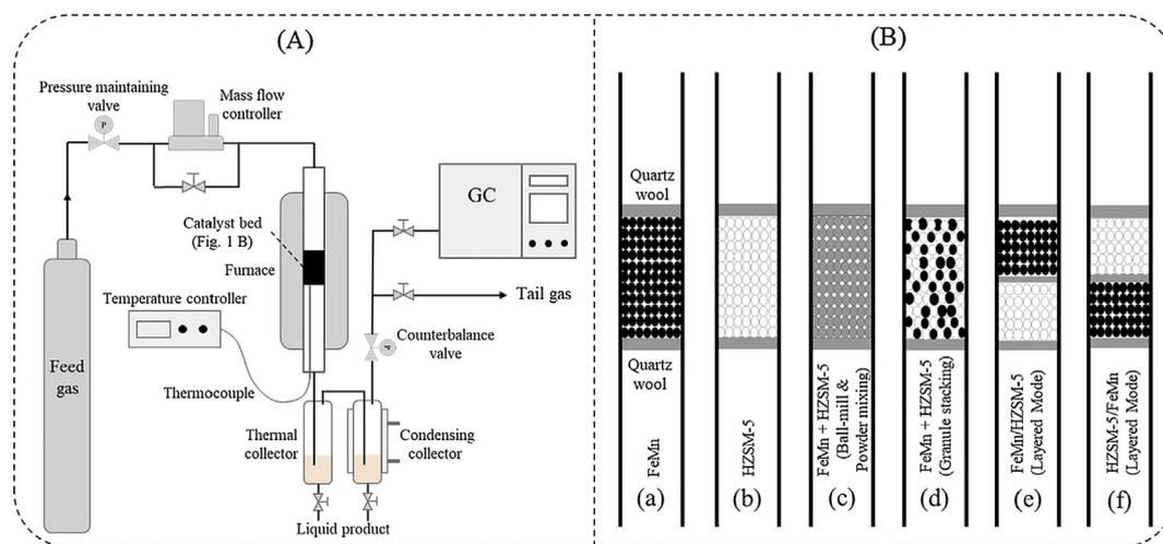
**Fig. 1.** Schematic experimental setup of the fixed-bed flowing reactor system for FT & Oli catalytic process (A) and different manners of the active components (B): (a) FT process on FeMn catalyst, (b) Oli process on HZSM-5 catalyst, (c) FT-Oli process on FeMn/HZSM-5-B or FeMn/HZSM-5-M (Ball-milling or Power-mixing configuration), (d) FT-Oli process on FeMn/HZSM-5-GS (Granule stacking configuration) and (e,f) FT-Oli process on FeMn/HZSM-5 or HZSM-5/FeMn (Dual-bed configuration).
